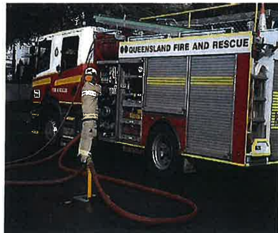
Figure 2 – Use of Hydrant System
