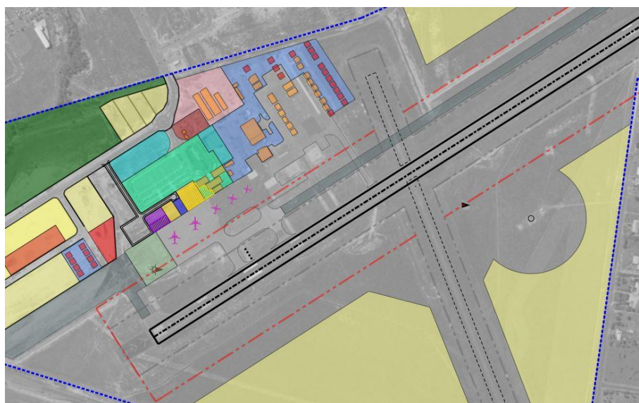
Figure 25: Indicative 300m runway strip alignment
