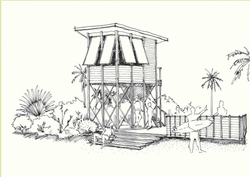
Figure 7—Proposed lookout tower—to be constructed on a retained portion of the SLSC floor slab after building demolition
