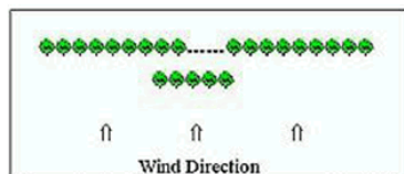
Figure 1. An island belt can prevent wind from tunneling through gaps within a shelterbelt
