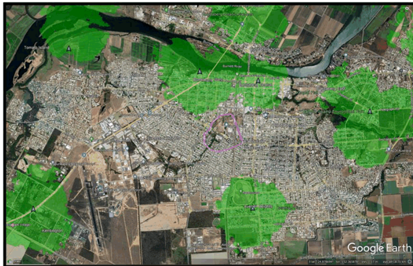
Figure 2: Existing 4G LTE1800 coverage in Bundaberg (green area) Target area for proposed facility is shown in pink
