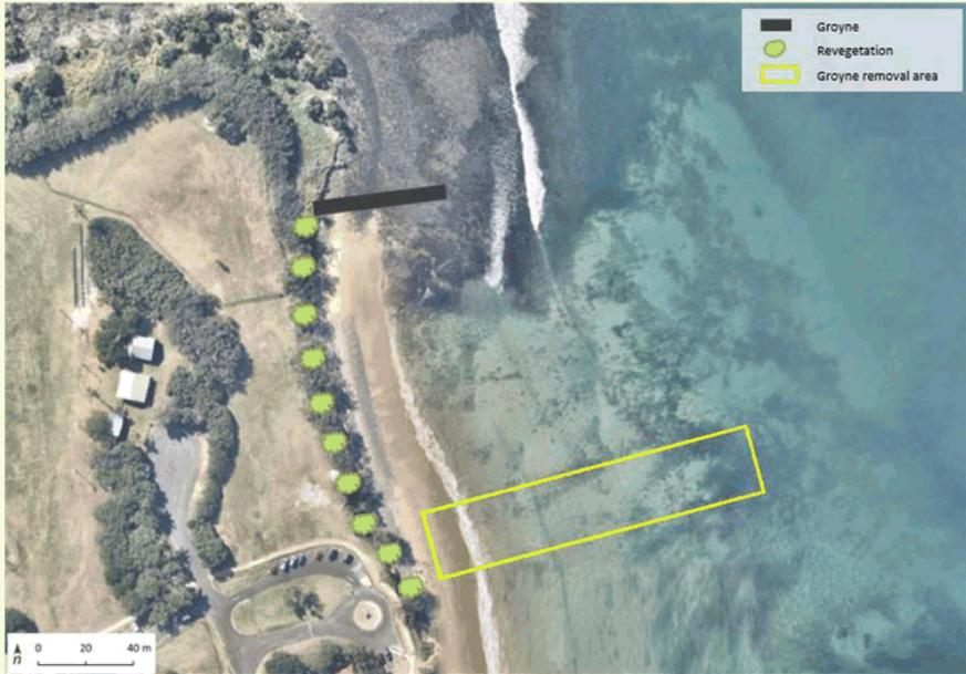
**Figure 35.** Jayteens Park - Option 5 – removal of existing groyne and construction new groyne.
