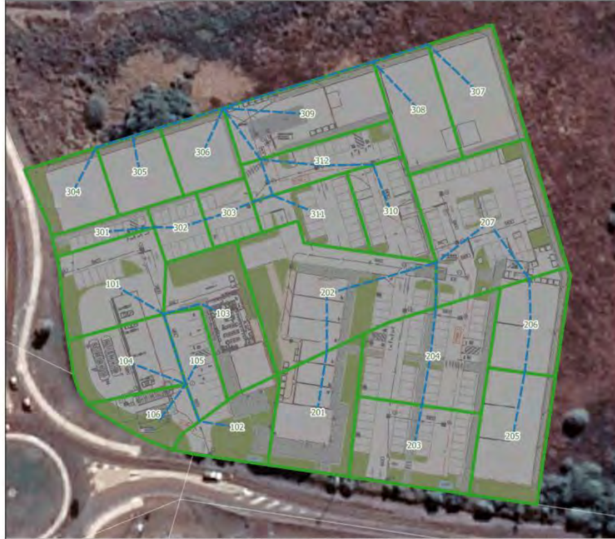
Figure 4.2 – Developed (Unmitigated) URBS Model Schematic
