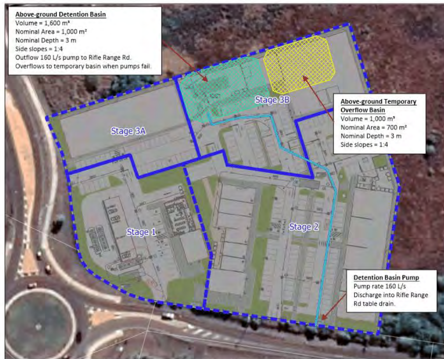
Figure 4.4 – Potential Location of Stormwater Basins
