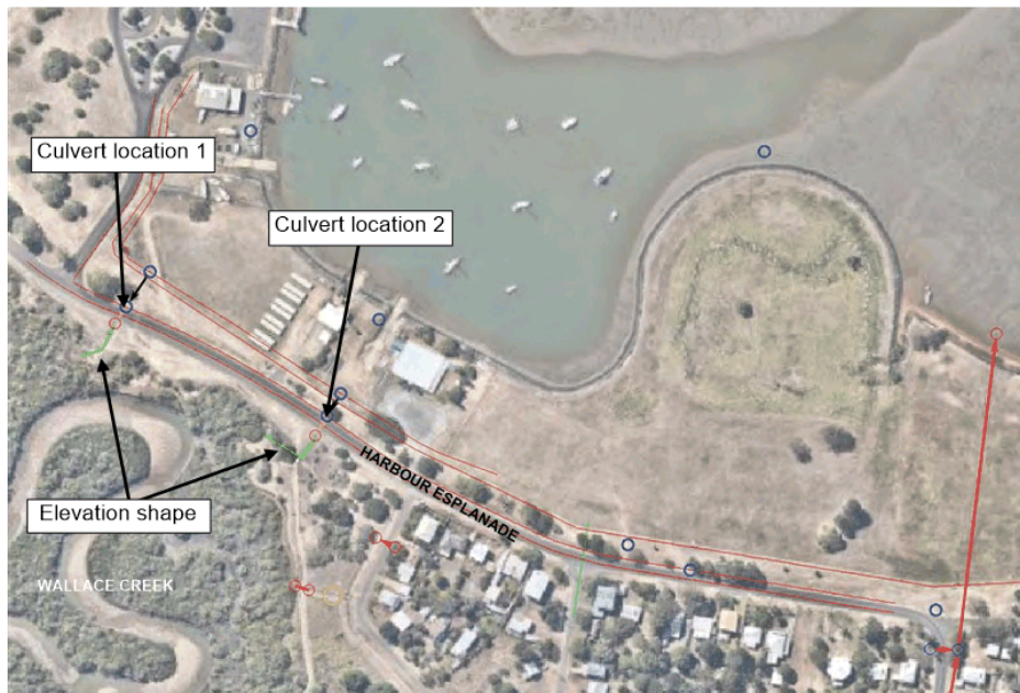
Figure 13: Culvert locations and elevation shapes
