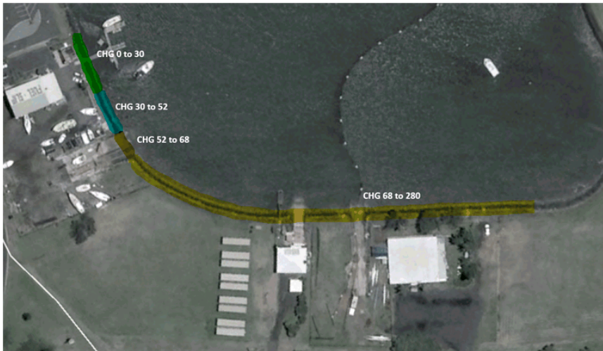
Figure 4 – Chainage Divisions for the Inspection
